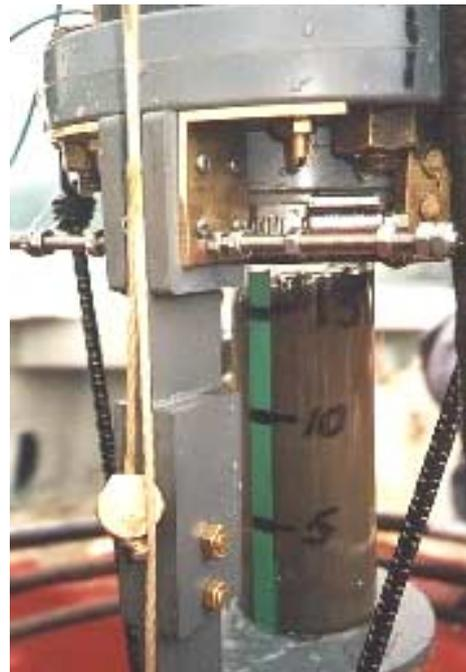
Figure 16. Sediment coring devices use to sample sediments in the Clyde sea area. a) Bowers & Connolly 4-channel multi-corer, b) multiple corer head, c) modified Craib corer c) high quality core sample taken by modified Craib core, the scale on the core tube showing depth of penetration (cm) into the sediment.
