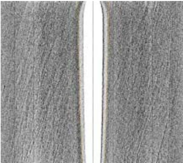
Figure 25. Along-track sidescan sonar image (Dia Island, Aegean Sea) recorded with towfish at 15 m above soft sea bed.
