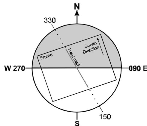
Figure 9. Schematic diagram illustrating how the orientation of a trawl mark can be described by one of two bearings (e.g.  $330^\circ$  or the reciprocal bearing  $150^\circ$ ). For surveys in the Clyde Sea area, bearings were standardised to have a southerly component (i.e. lie between  $090^\circ$  and  $270^\circ$ )
