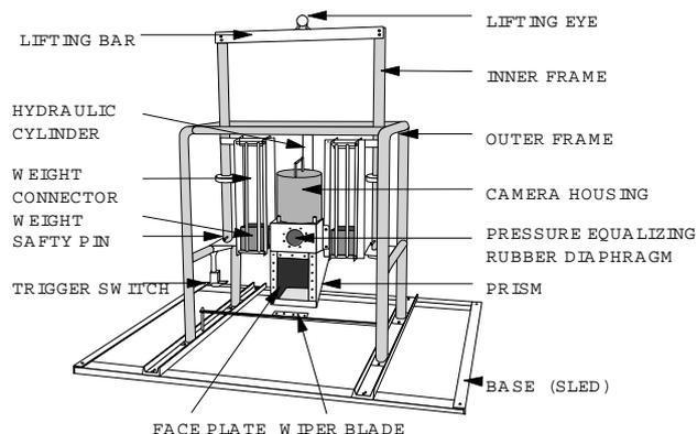
Figure 19. Schematic of the SPI system.
