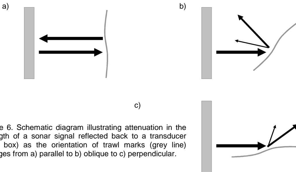
Figure 6. Schematic diagram illustrating attenuation in the strength of a sonar signal reflected back to a transducer (grey box) as the orientation of trawl marks (grey line) changes from a) parallel to b) oblique to c) perpendicular.
