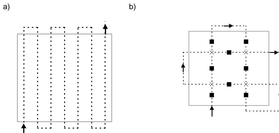
Figure 5. Stylised survey design for sidescan sonar surveys in the Clyde Sea area. a) a series of parallel passes, b) an open grid pattern from which 'snapshots' were taken. Filled squares represent 'frames', i.e. single snapshots. X represents 'intersects', i.e. paired frames taken at the same point but from perpendicular axes.
