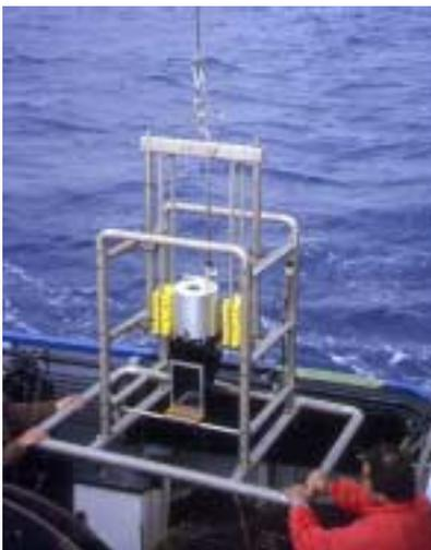
Figure 18. Photograph of the IMBC SPI system.
