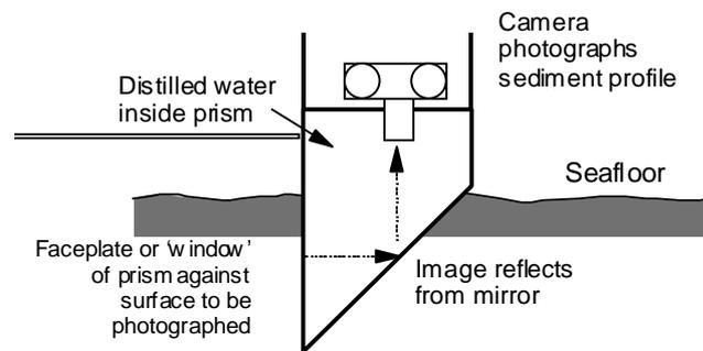
Figure 21. Schematic of prism operation.
