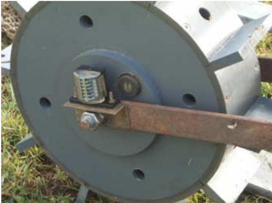
Figure 12. Odometer developed and tested by UMBSM for measuring distance covered by the 2-metre beam trawl. a) attached to the trawl frame, b) magnetically activated trip counter.
