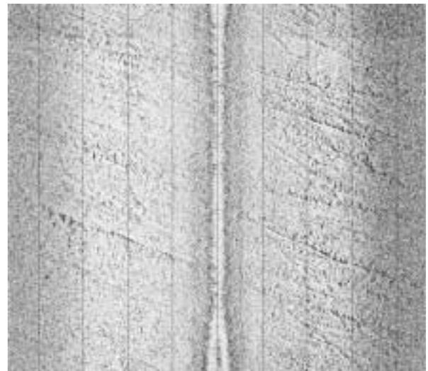
Figure 28. As Fig. 27 but with towfish ~ 5 m above soft sea bed.
