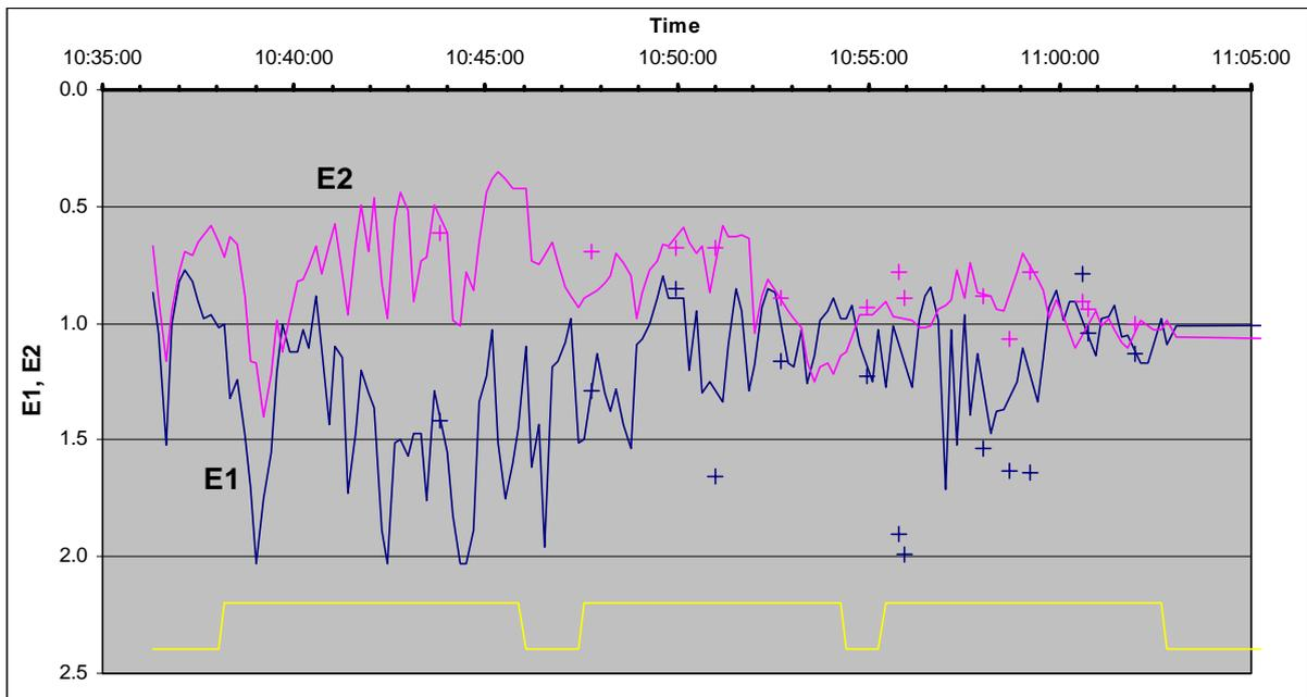
Figure 11. Illustration of the method for identifying anomalous data from the RoxAnn™ survey in the Clyde Sea area. Anomalous points are sought in the depth data (a) and their corresponding points in the E1 and E2 data (b) identified. These data are removed from the data set prior to analysis. For clarity of presentation, this example plots the anomalous data separately from cleaned data.
