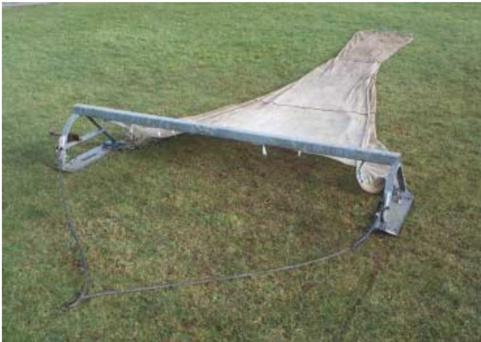
Figure 4. Small trawls used for sampling epibenthic megafauna. a) 2-metre Agassiz trawl (photo. courtesy of M. Bergmann), b) 2-metre beam trawl.
