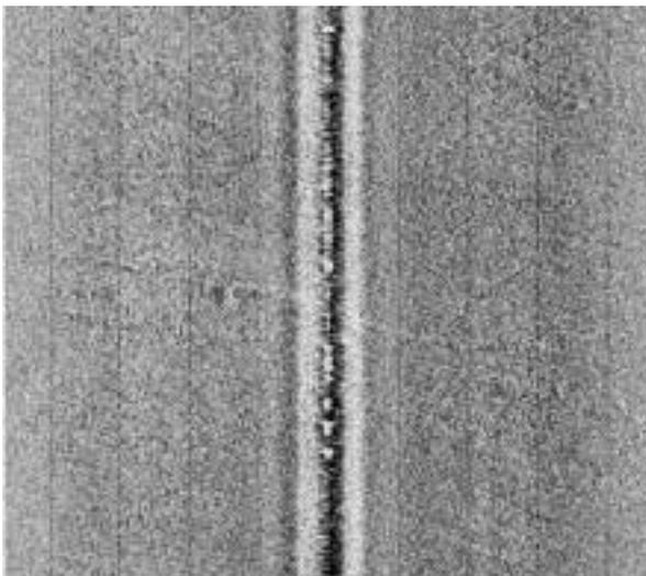
Figure 27. Cross-track sidescan sonar image (Dia Island, Aegean Sea) recorded with towfish ~ 10 m above soft sea bed.
