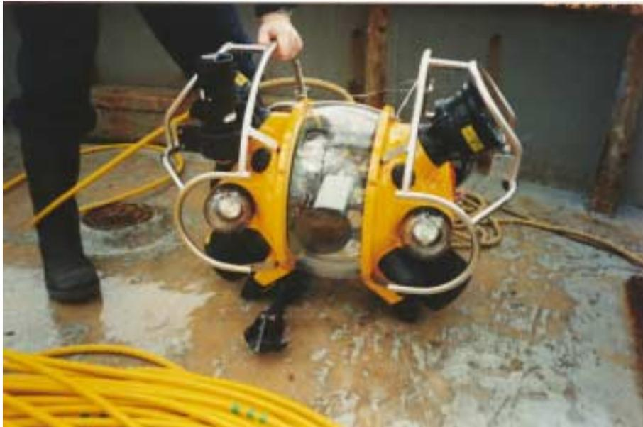
Figure 15. Equipment used for underwater television surveys in the Clyde Sea area. a) towed video-sledge, b) Hyball ROV (Hydrovision, Aberdeen, UK)
