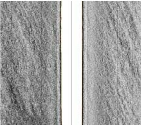
Figure 29. Diagonal-track sidescan sonar image (Gouves, Aegean Sea) recorded with towfish ~18 m above coarse sea bed.
