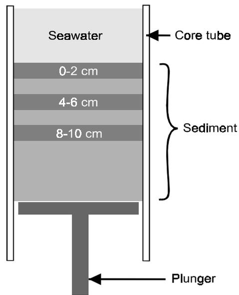
Figure 17. Schematic illustration of protocol for sampling three depth layers in sediment samples collected by coring in the Clyde Sea area (see text).
