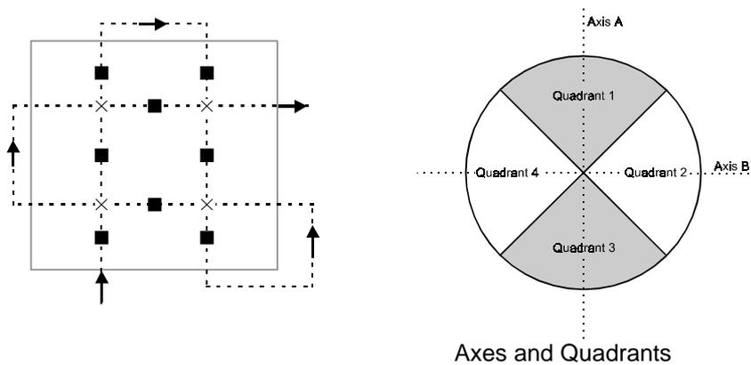
Figure 7. Schematic diagram explaining the nomenclature of Axes and Quadrants relative to the open grid survey pattern used in sidescan sonar surveys in the Clyde Sea area.
