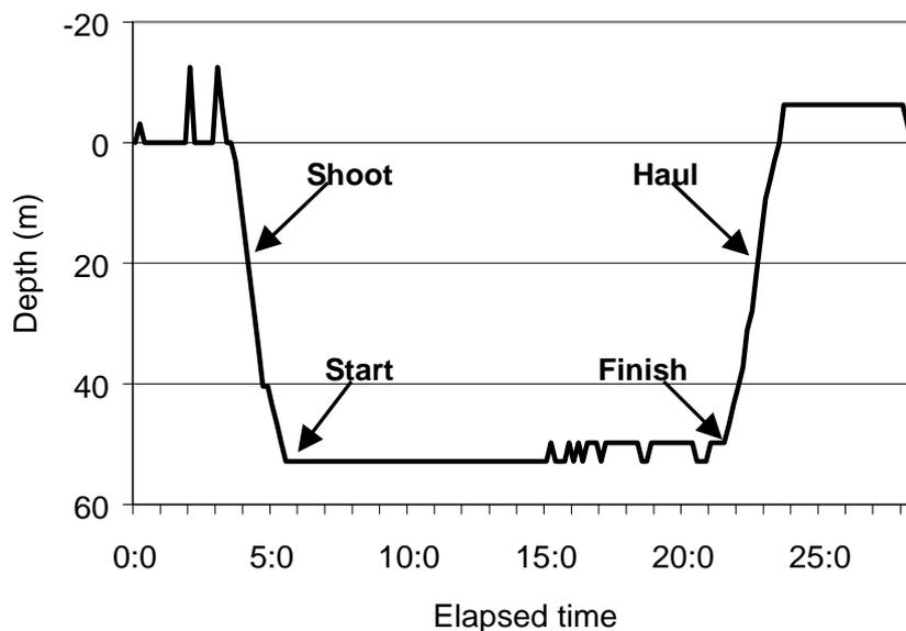
Figure 14. Example plot of time-depth data recorded by a Minilogger attached to the trawl gear used in the Clyde Sea area. The plot clearly shows when the trawl reached the sea bed after shooting, and when it left the sea bed on hauling
