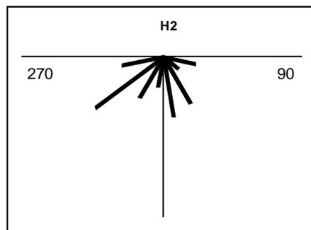
Figure 10. Illustration of plot used to visualise directional patterns in the trawl marks at a site surveyed by sidescan sonar using an open grid survey pattern.
