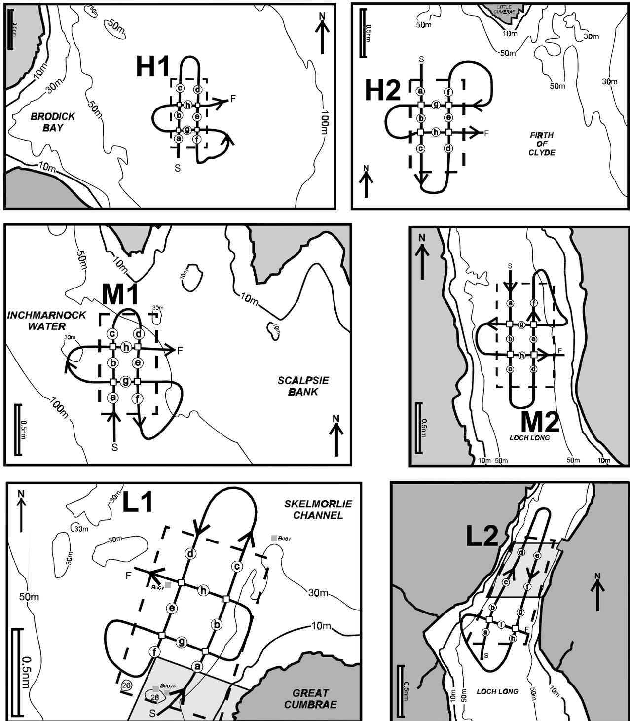
Figure 23. Charts indicating the tracks taken on the second sidescan sonar survey at each of the six sites in the Clyde Sea area. The dashed line shows the site boundary. Shaded areas in L1 and L2 indicate the zones in which trawling is prohibited. S and F indicate the start and finish of the survey track (respectively). Circled letters show the positions of the individual sonar snapshot 'frames'; the intersect snapshots were taken where the lines of the survey track cross (open squares).
