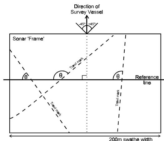
Figure 8. Schematic diagram illustrating the method for quantitative analysis of snapshot frames taken by sidescan sonar surveys in the Clyde Sea area.
